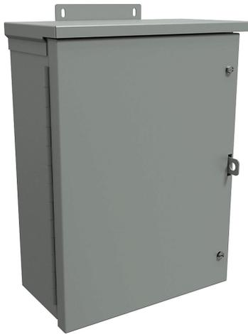
Hammond enclosure, NEMA 3R, 16 x 12 x 6in (HxWxD), wall mount, galvanized steel, ANSI 61 gray, powder coat finish, hinged screw cover, padlock hasp and staple.
