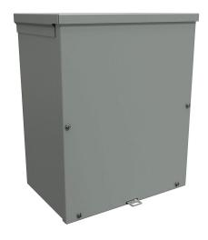
Hammond enclosure, NEMA 3R, 15 x 12 x 8in (HxWxD), wall mount, with knockouts, galvanized steel, ANSI 61 gray, powder coat finish, screw cover, padlock hasp and staple.
