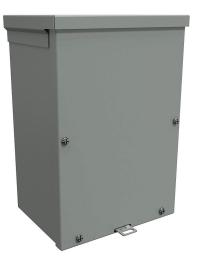
Hammond enclosure, NEMA 3R, 12 x 8 x 6in (HxWxD), wall mount, with knockouts, galvanized steel, ANSI 61 gray, powder coat finish, screw cover, padlock hasp and staple.
