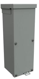
Hammond enclosure, NEMA 3R, 12 x 4 x 4in (HxWxD), wall mount, with knockouts, galvanized steel, ANSI 61 gray, powder coat finish, screw cover, padlock hasp and staple.
