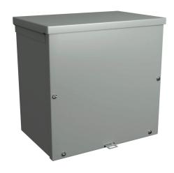
Hammond enclosure, NEMA 3R, 12 x 12 x 8in (HxWxD), wall mount, galvanized steel, powder coat finish, screw cover, padlock hasp and staple.
