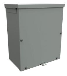
Hammond enclosure, NEMA 3R, 12 x 10 x 6in (HxWxD), wall mount, with knockouts, galvanized steel, ANSI 61 gray, powder coat finish, screw cover, padlock hasp and staple.
