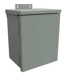
Hammond enclosure, NEMA 3R, 10 x 8 x 6in (HxWxD), wall mount, with knockouts, galvanized steel, ANSI 61 gray, powder coat finish, single-door, quick-release latch, padlock hasp and staple.
