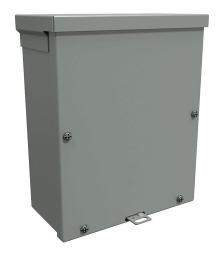
Hammond enclosure, NEMA 3R, 10 x 8 x 4in (HxWxD), wall mount, with knockouts, galvanized steel, ANSI 61 gray, powder coat finish, screw cover, padlock hasp and staple.
