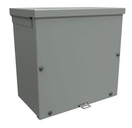
Hammond enclosure, NEMA 3R, 10 x 10 x 6in (HxWxD), wall mount, with knockouts, galvanized steel, ANSI 61 gray, powder coat finish, screw cover, padlock hasp and staple.
