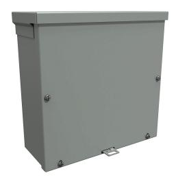
Hammond enclosure, NEMA 3R, 10 x 10 x 4in (HxWxD), wall mount, with knockouts, galvanized steel, ANSI 61 gray, powder coat finish, screw cover, padlock hasp and staple.
