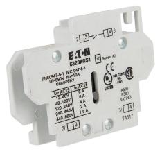
Eaton auxiliary contact, side mount, (1) N.O. contact(s), 6A @ 120 VAC/1.1A @ 120 VDC. For use with Cutler-Hammer AE series starters and CE series contactors.
