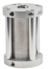
NITRA pneumatic cylinder, compact, 2in bore, 3/4in rod diameter, 3-1/2in stroke, double acting, counter-bored holes mount.
