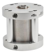
NITRA pneumatic cylinder, compact, 2in bore, 3/4in rod diameter, 2in stroke, double acting, counter-bored holes mount.
