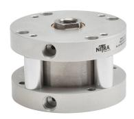
NITRA pneumatic cylinder, compact, 2in bore, 3/4in rod diameter, 1in stroke, double acting, counter-bored holes mount.
