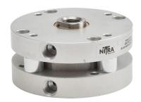
NITRA pneumatic cylinder, compact, 2in bore, 3/4in rod diameter, 1/2in stroke, double acting, counter-bored holes mount.
