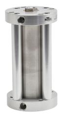
NITRA pneumatic cylinder, compact, 1-1/2in bore, 5/8in rod diameter, 4in stroke, double acting, counter-bored holes mount.
