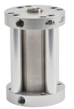
NITRA pneumatic cylinder, compact, 1-1/2in bore, 5/8in rod diameter, 3in stroke, double acting, counter-bored holes mount.
