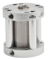
NITRA pneumatic cylinder, compact, 1-1/2in bore, 5/8in rod diameter, 2in stroke, double acting, counter-bored holes mount.
