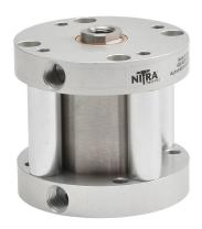
NITRA pneumatic cylinder, compact, 1-1/2in bore, 5/8in rod diameter, 1-1/2in stroke, double acting, counter-bored holes mount.
