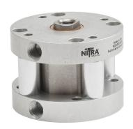
NITRA pneumatic cylinder, compact, 1-1/2in bore, 5/8in rod diameter, 1in stroke, double acting, counter-bored holes mount.
