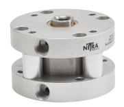
NITRA pneumatic cylinder, compact, 1-1/2in bore, 5/8in rod diameter, 3/4in stroke, double acting, counter-bored holes mount.
