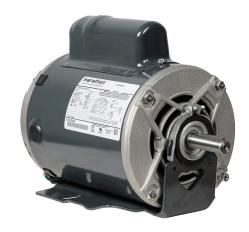
Marathon standard efficiency AC induction motor, fan and blower, 1hp, 1-phase, 115/208-230 VAC, 1800rpm, ODP, NEMA 56 frame, rolled steel, resilient base mount.
