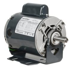
Marathon standard efficiency AC induction motor, fan and blower, 1/3hp, 1-phase, 115/208-230 VAC, 1800rpm, ODP, NEMA 56 frame, rolled steel, resilient base mount.
