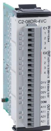
CLICK PLUS discrete/analog combo module, Analog Input: 2-channel, current/voltage, Analog Output: 2-channel, current/voltage, Discrete Input: 4-point, sinking/sourcing, Discrete Output: 4-point, relay, (4) Form A (SPST) relays.
