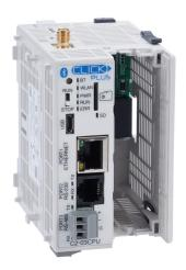
CLICK PLUS PLC, 24 VDC required, (1) option slot, WiFi LAN/Bluetooth, Ethernet, serial and microB-USB ports, microSD card slot, no on-board I/O.
