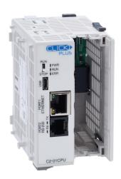
CLICK PLUS PLC, 24 VDC required, (1) option slot, Ethernet, serial and microB-USB ports, no on-board I/O.
