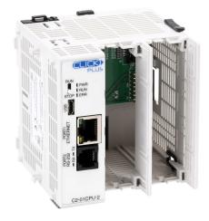
CLICK PLUS PLC, 24 VDC required, (2) option slots, Ethernet, serial and microB-USB ports, no on-board I/O.
