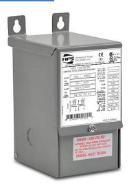
Hammond general purpose transformer, encapsulated core, 250 VA, 1-phase, 190/200/208/220/240 or 380/400/416/440/480 VAC primary, 120/240 VAC secondary, 50/60 Hz, NEMA 3R, wall mount.
