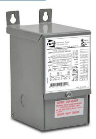
Hammond general purpose transformer, encapsulated core, 250 VA, 1-phase, 120/208/240/277 VAC primary, 120/240 VAC secondary, 60 Hz, NEMA 3R, wall mount.
