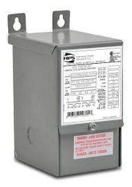
Hammond general purpose transformer, encapsulated core, 100 VA, 1-phase, 120/208/240/277 VAC primary, 120/240 VAC secondary, 60 Hz, NEMA 3R, wall mount.
