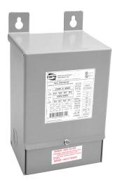
Hammond general purpose transformer, encapsulated core, 1.5 kVA, 1-phase, 240/480 VAC primary, 120/240 VAC secondary, 60 Hz, electrostatic shield, NEMA 3R, wall mount.
