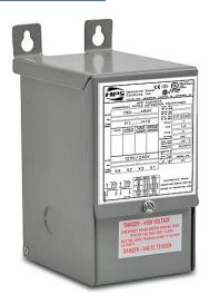
Hammond general purpose transformer, encapsulated core, 1 kVA, 1-phase, 190/200/208/220/240 or 380/400/416/440/480 VAC primary, 120/240 VAC secondary, 50/60 Hz, electrostatic shield, NEMA 3R, wall mount.
