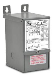
Hammond general purpose transformer, encapsulated core, 1 kVA, 1-phase, 120/208/240/277 VAC primary, 120/240 VAC secondary, 60 Hz, electrostatic shield, NEMA 3R, wall mount.
