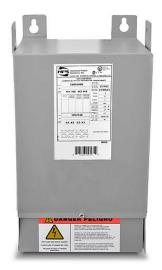
Hammond general purpose transformer, encapsulated core, 15 kVA, 1-phase, 240/480 VAC primary, 120/240 VAC secondary, 60 Hz, electrostatic shield, NEMA 3R, wall mount.
