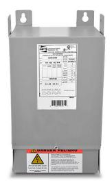
Hammond general purpose transformer, encapsulated core, 10 kVA, 1-phase, 240/480 VAC primary, 120/240 VAC secondary, 60 Hz, electrostatic shield, NEMA 3R, wall mount.
