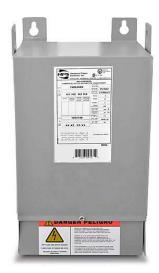
Hammond general purpose transformer, encapsulated core, 10 kVA, 1-phase, 240/480 VAC primary, 120/240 VAC secondary, 60 Hz, electrostatic shield, NEMA 3R, wall mount.
