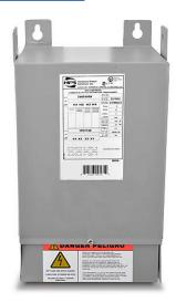
Hammond general purpose transformer, encapsulated core, 7.5 kVA, 1-phase, 240/480 VAC primary, 120/240 VAC secondary, 60 Hz, electrostatic shield, NEMA 3R, wall mount.
