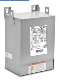
Hammond general purpose transformer, encapsulated core, 5 kVA, 1-phase, 190/200/208/220/240 or 380/400/416/440/480 VAC primary, 120/240 VAC secondary, 50/60 Hz, electrostatic shield, NEMA 3R, wall mount.
