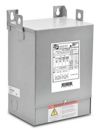
Hammond general purpose transformer, encapsulated core, 5 kVA, 1-phase, 120/208/240/277 VAC primary, 120/240 VAC secondary, 60 Hz, electrostatic shield, NEMA 3R, wall mount.
