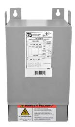
Hammond general purpose transformer, encapsulated core, 5 kVA, 1-phase, 240/480 VAC primary, 120/240 VAC secondary, 60 Hz, electrostatic shield, NEMA 3R, wall mount.
