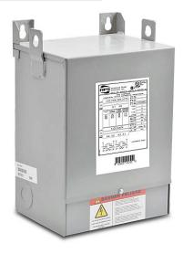
Hammond general purpose transformer, encapsulated core, 3 kVA, 1-phase, 120/208/240/277 VAC primary, 120/240 VAC secondary, 60 Hz, electrostatic shield, NEMA 3R, wall mount.
