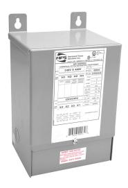
Hammond general purpose transformer, encapsulated core, 3 kVA, 1-phase, 240/480 VAC primary, 120/240 VAC secondary, 60 Hz, electrostatic shield, NEMA 3R, wall mount.
