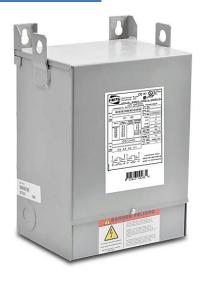
Hammond general purpose transformer, encapsulated core, 2 kVA, 1-phase, 190/200/208/220/240 or 380/400/416/440/480 VAC primary, 120/240 VAC secondary, 50/60 Hz, electrostatic shield, NEMA 3R, wall mount.
