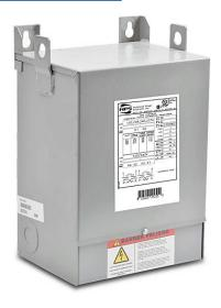
Hammond general purpose transformer, encapsulated core, 2 kVA, 1-phase, 120/208/240/277 VAC primary, 120/240 VAC secondary, 60 Hz, electrostatic shield, NEMA 3R, wall mount.
