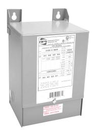
Hammond general purpose transformer, encapsulated core, 2 kVA, 1-phase, 240/480 VAC primary, 120/240 VAC secondary, 60 Hz, electrostatic shield, NEMA 3R, wall mount.
