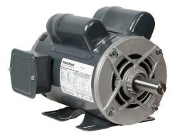
Marathon standard efficiency AC induction motor, general purpose, 3hp, 1-phase, 115/230 VAC, 3600rpm, ODP, NEMA 145T frame, rolled steel, rigid base mount.
