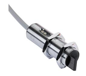
AutomationDirect photoelectric sensor, tubular, threaded, metal housing, through-beam receiver, right-angle lens, 6m sensing distance, 10-36 VDC operating voltage, complementary light-on/dark-on, PNP, 4-wire, pigtail.
