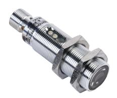
AutomationDirect photoelectric sensor, tubular, threaded, metal housing, through-beam receiver, 6m sensing distance, 10-36 VDC operating voltage, complementary light-on/dark-on, PNP, 4-wire, 4-pin M12 quick-disconnect.
