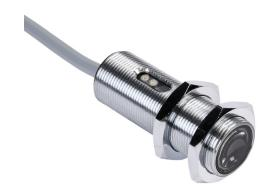
AutomationDirect photoelectric sensor, tubular, threaded, metal housing, through-beam receiver, 6m sensing distance, 10-36 VDC operating voltage, complementary light-on/dark-on, PNP, 4-wire, pigtail.
