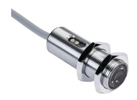
AutomationDirect photoelectric sensor, tubular, threaded, metal housing, through-beam receiver, 6m sensing distance, 10-36 VDC operating voltage, complementary light-on/dark-on, PNP, 4-wire, pigtail.
