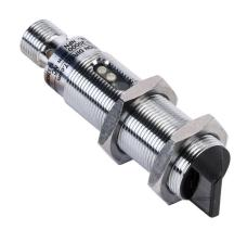
AutomationDirect photoelectric sensor, tubular, threaded, metal housing, through-beam receiver, right-angle lens, 6m sensing distance, 10-36 VDC operating voltage, complementary light-on/dark-on, NPN, 4-wire, 4-pin M12 quick-disconnect.
