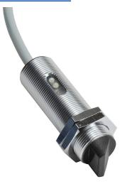
AutomationDirect photoelectric sensor, tubular, threaded, metal housing, through-beam receiver, right-angle lens, 6m sensing distance, 10-36 VDC operating voltage, complementary light-on/ dark-on, NPN, 4-wire, pigtail.
